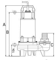
unit : mm C.W.L : Continuous running water level L.W.L : Lowest running water level
